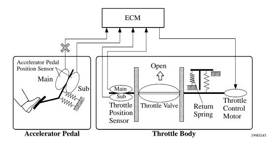
• If both circuits have a malfunction, the ECM detects the abnormal signal by voltage from these two sensor circuits and discontinues the throttle control. At this time, the vehicle can be driven within its idling range.
